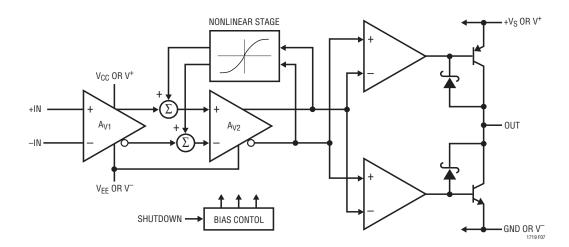
Figure 7. LT1719 Block Diagram
