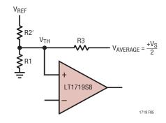
Figure 5. Model for Additional Hysteresis Calculations
