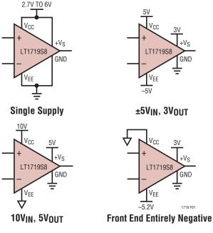
Figure 1. Variety of SO-8 Power Supply Configurations
