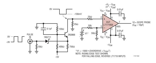
±V<sub>TRIP</sub> Test Circuit
