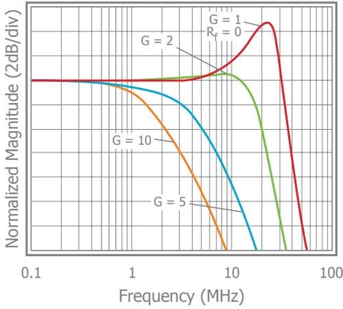
Inverting Frequency Response at  $V_S = 5\text{V}$
