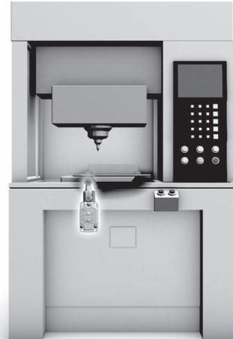
**Detection of Forward and Reverse Movement of Hydraulic Cylinders on Molding Machines**
