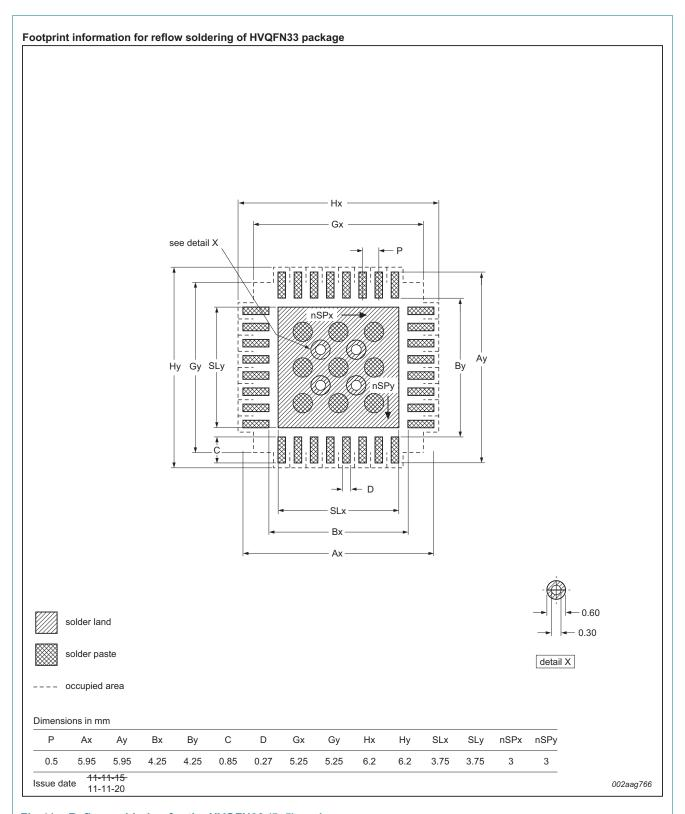
Fig 41. Reflow soldering for the HVQFN33 (5x5) package
