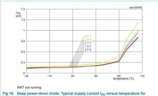
different supply voltages V<sub>DD</sub>
