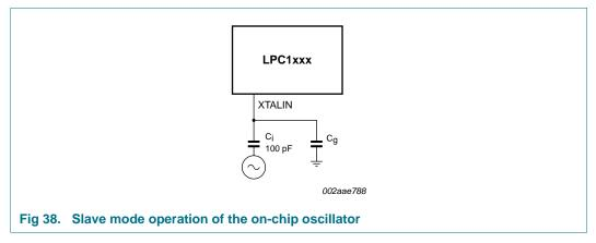
In slave mode the input clock signal should be coupled through a capacitor of 100 pF ( $\underline{Figure 38}$ ), with an amplitude between 200 mV (RMS) and 1000 mV (RMS). This corresponds to a square wave signal with a signal swing of between 280 mV and 1.4 V. The XTALOUT pin in this configuration can be left unconnected.
