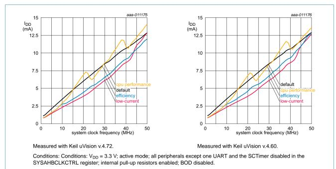
Fig 22. Active mode: CoreMark power consumption I<sub>DD</sub> for different power mode settings of the power profiles
