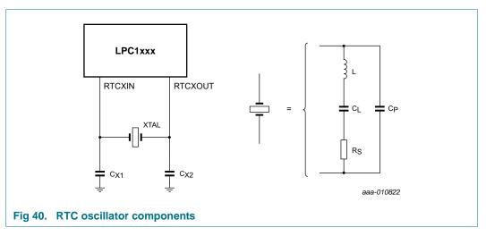
Select  $C_{x1}$  and  $C_{x2}$  based on the external 32 kHz crystal used in the application circuitry. The pad capacitance  $C_P$  of the RTCXIN and RTCXOUT pad is 3 pF. If load capacitance of the external crystal is  $C_L$ , the optimal  $C_{x1}$  and  $C_{x2}$  can be selected as:
