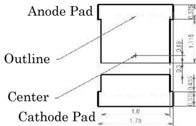
Mountability and solderability need to be optimized with actual conditions such as amount of solder, reflow temperature applied in the process.
