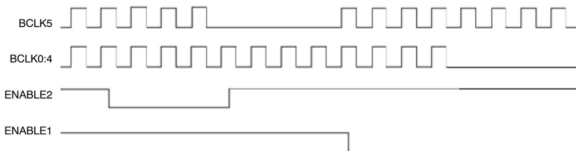
**Figure 3. ENABLEx Control Timing Diagram**
