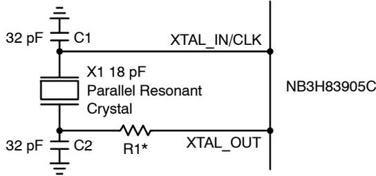
**Figure 8. NB3H83905C Crystal Oscillator Interface**
