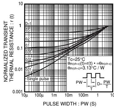
Fig.14 Normalized Transient Thermal Resistance vs. Pulse Width
