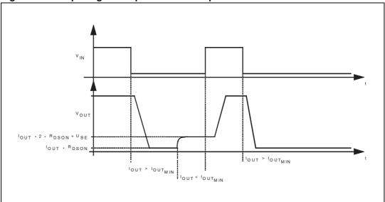
Figure 5. Output signal shape related to output current
