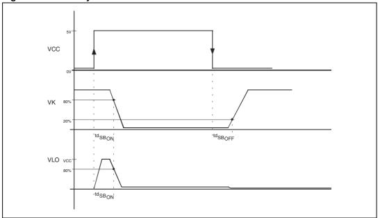
Figure 8. Standby current consumption
