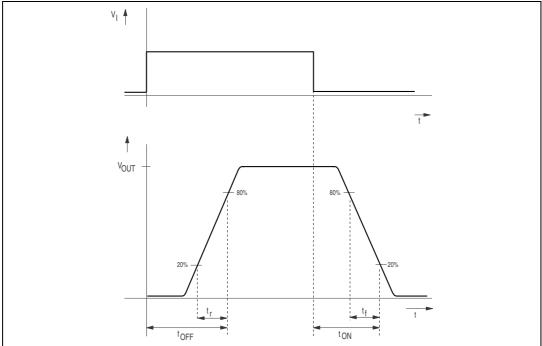
Figure 7. Standby reaction time
