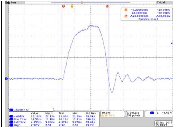
PCO-7121 (50 A, 22 ns, shorted load, inverted waveform)
