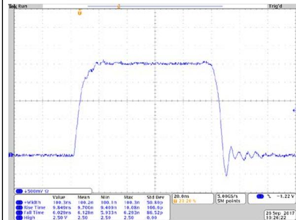
PCO-7121 (50 A, 100 ns, shorted load, inverted waveform)
