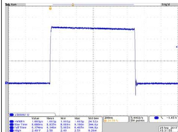
PCO-7121 (50 A, 1000 ns, shorted load, inverted waveform)
