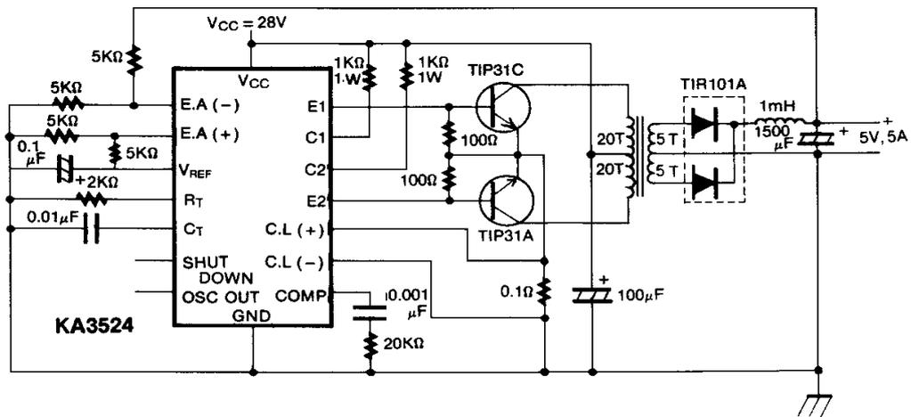
Figure 12. Push-pull Transformer-coupled Circuit
