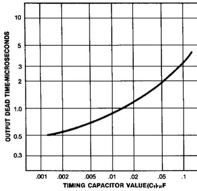
Figure 6. Output Stage Dead Time As A Function
