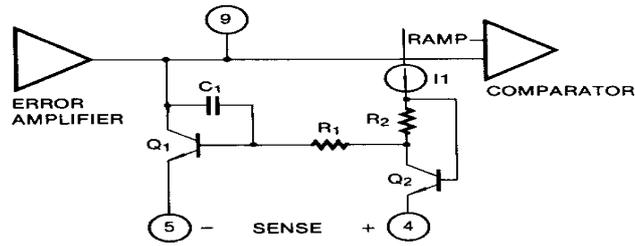
Figure 4. Current Limiting Circuit Of The Ka3524
