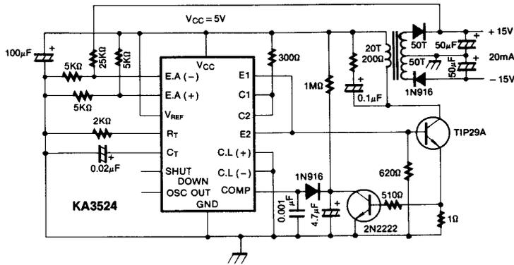
Figure 10. Flyback Converter Circuit
