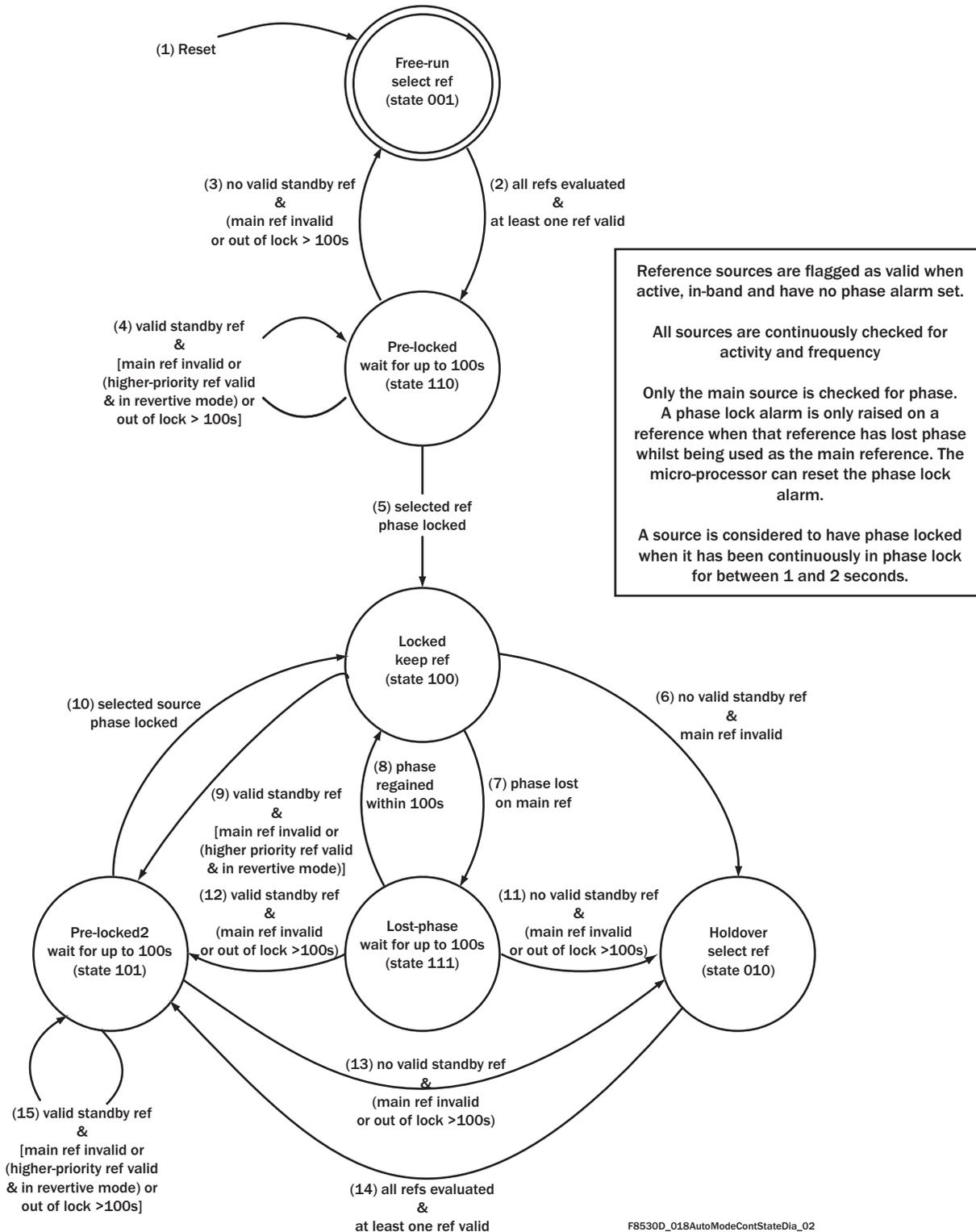
Note...The state diagram above is for T0 DPLL only, and the 3-bit state value refers to the register `sts_operating Reg. 09 Bits [2:0] T0_DPLL_operating_mode`. By contrast, the T4 DPLL has only automatic operation and can be in one of only two possible states: "Instantaneous Holdover" with zero frequency offset (its start-up state), or "Locked". The T4 DPLL states are not configurable by the User and there is no "Free-run" state.
