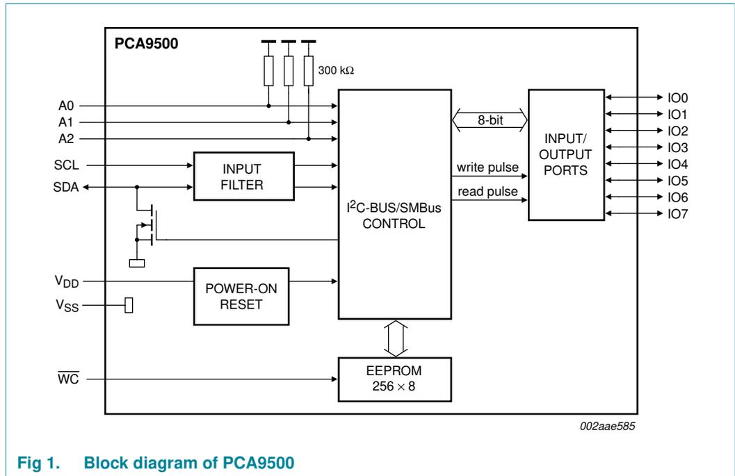
Fig 1. Block diagram of PCA9500
