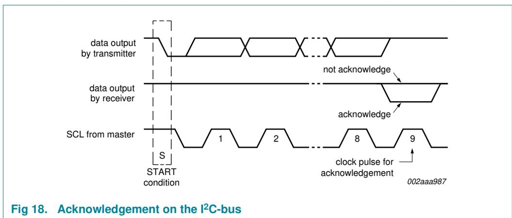
Fig 18. Acknowledgement on the I<sup>2</sup>C-bus
