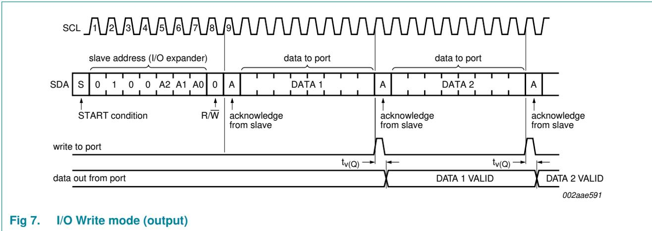
Fig 7. I/O Write mode (output)
