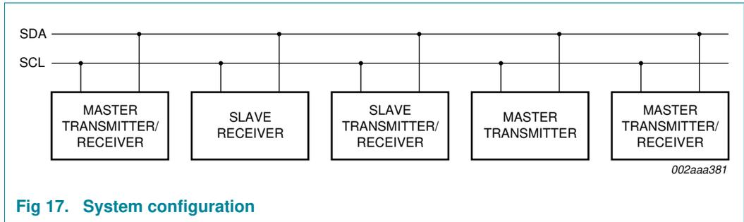
Fig 17. System configuration
