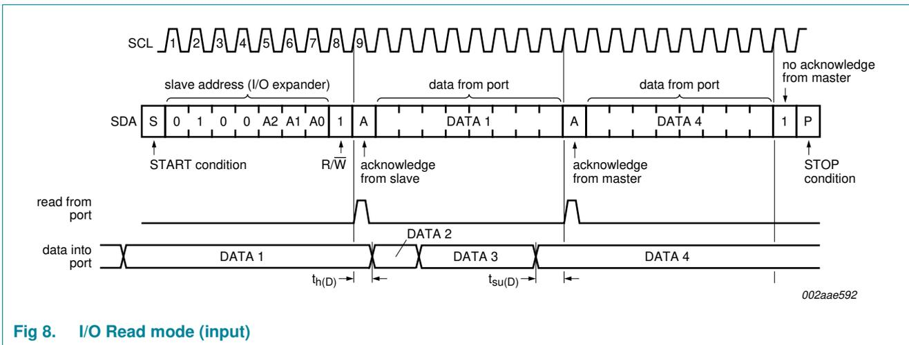
Fig 8. I/O Read mode (input)
