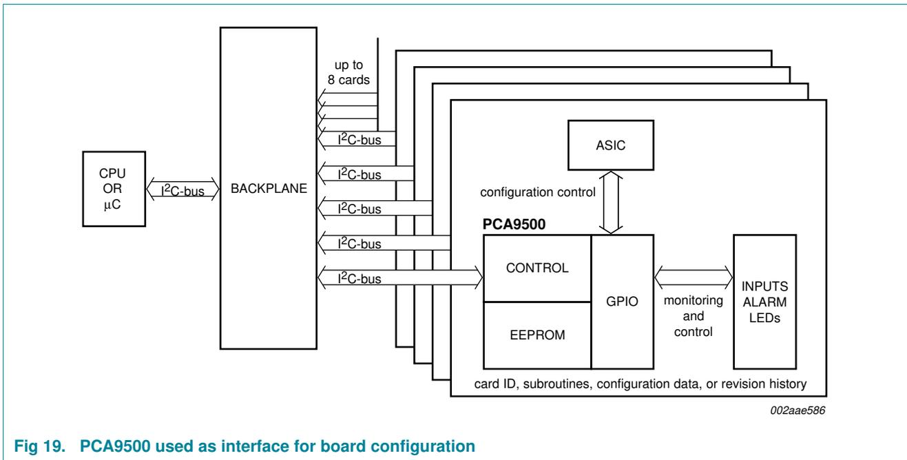
Fig 19. PCA9500 used as interface for board configuration
