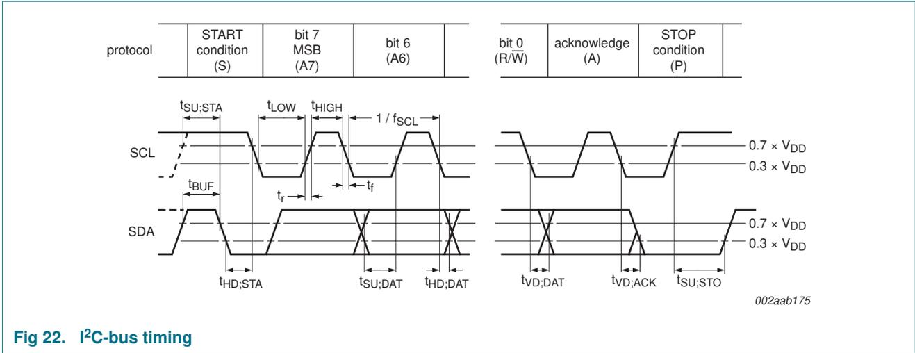
Fig 22. I<sup>2</sup>C-bus timing
