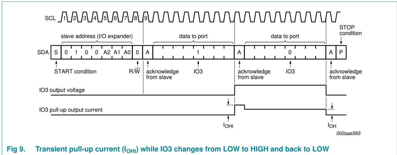
Fig 9. Transient pull-up current (I<sub>OHt</sub>) while IO3 changes from LOW to HIGH and back to LOW
