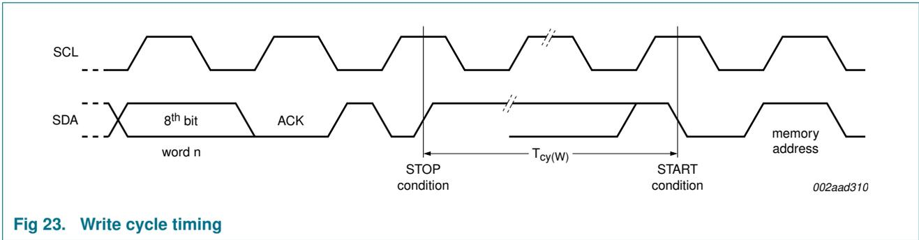
Fig 23. Write cycle timing
