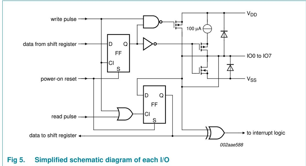
**Fig 5. Simplified schematic diagram of each I/O**
