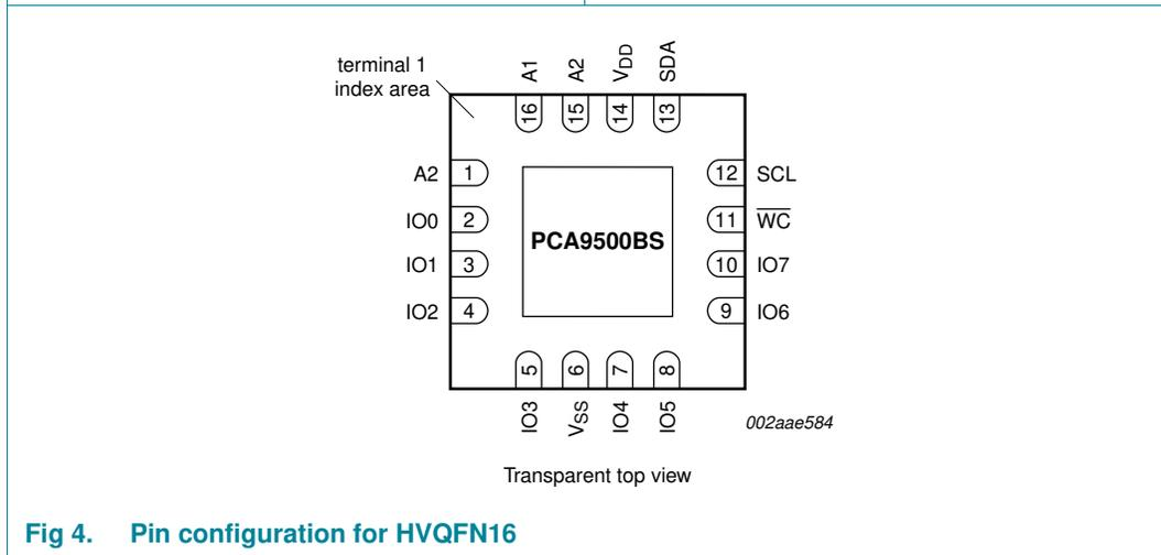
Fig 4. Pin configuration for HVQFN16
