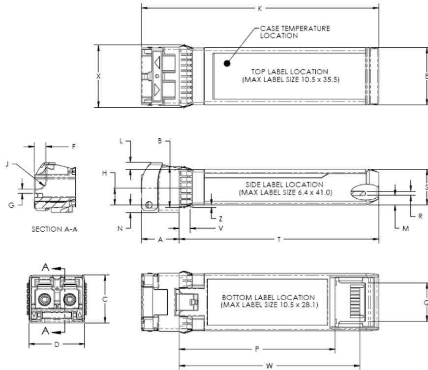
Figure 2. Mechanical Dimensions
