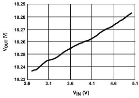
FIGURE 10. LINE REGULATION (I<sub>OUT</sub> = 30mA)
