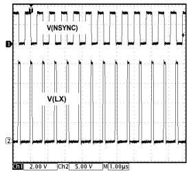
FIGURE 17. LX SYNCHRONIZATION WITH f(SYNC) = 1.4MHz
