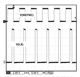
FIGURE 16. LX SYNCHRONIZATION WITH f(SYNC) = 600kHz
