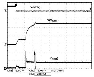
FIGURE 6. START-UP TO 12V ( $V_{DD}$  = 3.6V,  $R_L$  = 360 $\Omega$ )
