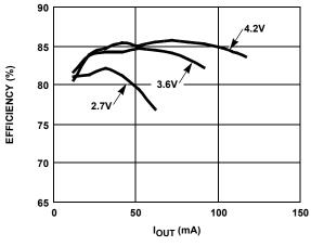
FIGURE 3. EFFICIENCY vs  $I_{OUT}$  ( $V_{OUT}$  = 18.3V) L = 6.8µH (TDK RLF7030) C = 6.6µF
