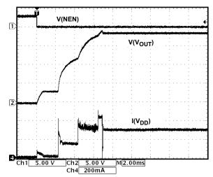
FIGURE 7. START-UP TO 18V ( $V_{DD}$  = 3.6V,  $R_L$  = 360 $\Omega$ )
