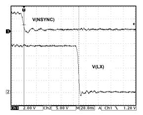
FIGURE 15. NSYNC TO LX SYNCHRONIZATION DELAY
