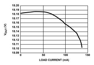
FIGURE 9. LOAD REGULATION ( $V_{IN} = 3.6V$ )
