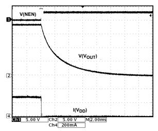
FIGURE 8. SHUTDOWN ( $V_{DD} = 3.6V$ ,  $R_L = 360\Omega$ )
