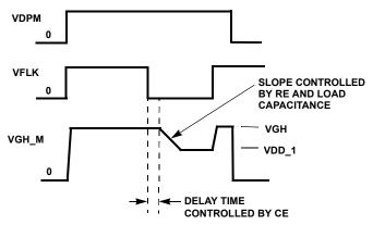
FIGURE 17. GATE PULSE MODULATOR TIMING DIAGRAM
