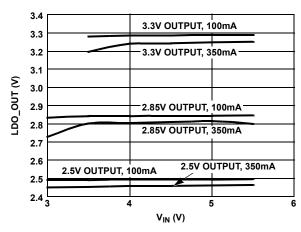
FIGURE 5. LINE REGULATION LDO\_OUT vs VIN
