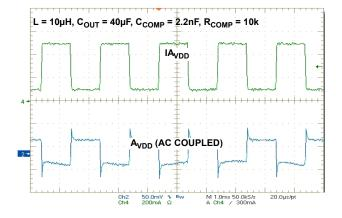
FIGURE 4. BOOST CONVERTER TRANSIENT RESPONSE
