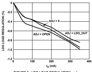
FIGURE 6. LDO LOAD REGULATION vs IO
