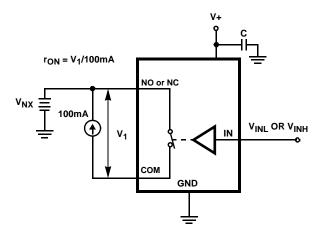
FIGURE 4. ron TEST CIRCUIT
