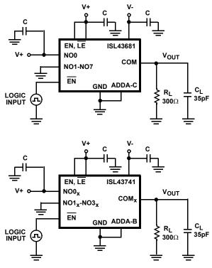
Repeat test for other switches.  $C_L$  includes fixture and stray capacitance.
