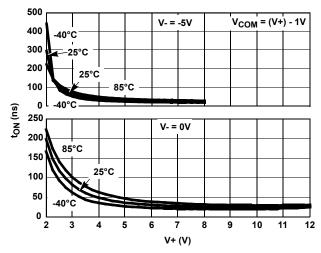
FIGURE 14. ENABLE TURN - ON TIME vs SUPPLY VOLTAGE
