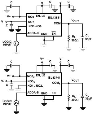
Repeat test for other switches. C<sub>L</sub> includes fixture and stray capacitance.
