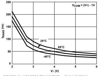
FIGURE 17. ADDRESS TRANS TIME vs DUAL SUPPLY VOLTAGE
