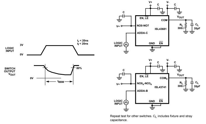
FIGURE 3A. tBBM MEASUREMENT POINTS
