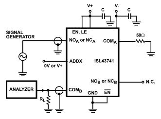
FIGURE 7. CROSSTALK TEST CIRCUIT
