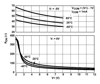
FIGURE 10. ON RESISTANCE vs SUPPLY VOLTAGE
