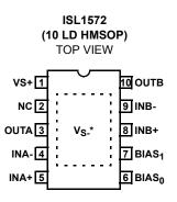
\*THERMAL PAD MUST BE CONNECTED TO NEGATIVE SUPPLY:  $\rm V_{S\_}.$  HMSOP PACKAGE CAN BE USED IN SINGLE SUPPLY APPLICATIONS ONLY.
