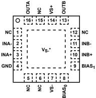
\*THERMAL PAD MUST BE CONNECTED TO NEGATIVE SUPPLY:  $\mathsf{V}_{S}\mathsf{.}$  . QFN PACKAGE CAN BE USED IN SINGLE AND DUAL SUPPLY APPLICATIONS.
