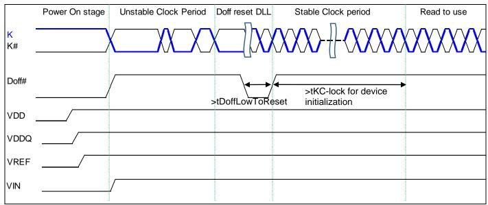
Note) Applying DLL reset sequences (sequence 3a, 3b) are also required when operating frequency is changed without power off. Note) All inputs including clocks must be either logically High or Low during Power On stage. Timing above shows only one of cases.
