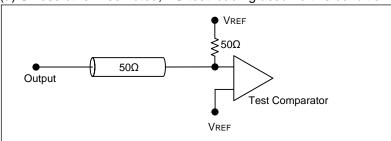
(b) tCHQZ and tCHQX1 are specified with 5pF load capacitance and measured when transition occurs ±100mV from the steady state voltage.
