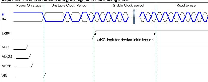
Note) All inputs including clocks must be either logically High or Low during Power On stage. Timing above shows only one of cases.
