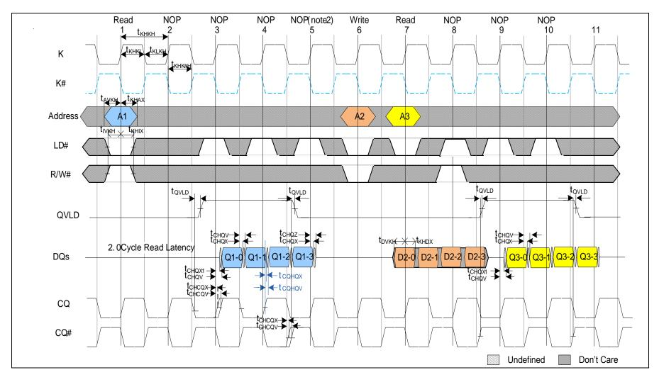
Notes: 1. Q1-0 refers to the output from address A1. Q1-1,Q1-2, and Q1-3 refer to the output from the next burst address following A1.
