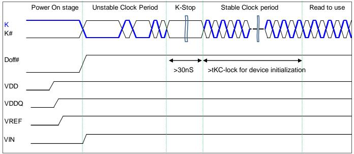
Note) All inputs including clocks must be either logically High or Low during Power On stage. Timing above shows only one of cases.
