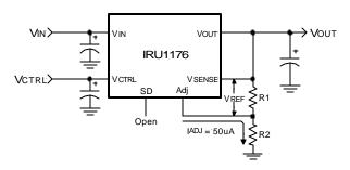
Figure 3 - Typical application of the IRU1176 for programming the output voltage.
