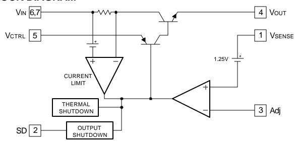
Figure 2 - Simplified block diagram of the IRU1176.
