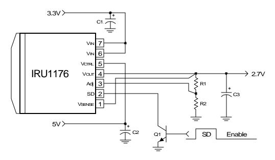
Figure 1 - Typical application of IRU1176.
