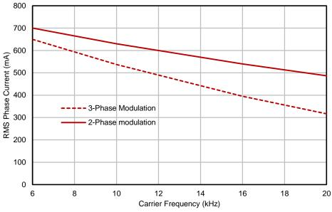
Figure 6: Maximum sinusoidal phase current vs PWM switching frequency, no heat sink. Space Vector Modulation, V+=320V,  $T_A$ =28°C,  $T_J$ =128°C
