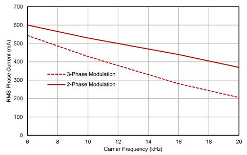
Figure 7: Maximum sinusoidal phase current vs PWM switching frequency, no heat sink. Space Vector Modulation, V+=320V, T<sub>A</sub>=28°C, T<sub>J</sub>=98°C
