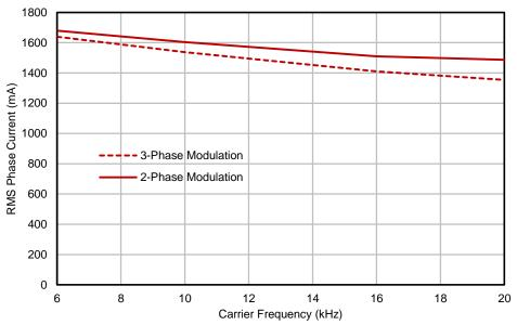
**Figure 5:** Maximum sinusoidal phase current vs PWM switching frequency with a heat sink. Space Vector Modulation, V+=320V, T<sub>A</sub>=28°C, T<sub>J</sub>=150°C, T<sub>C</sub>=125°C
