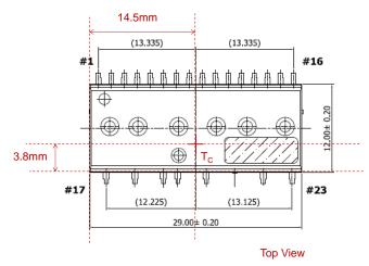
Figure 2: T<sub>C</sub> measurement point for R<sub>th(j-C)</sub>
