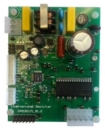
Figure 4: Reference design board featuring the µIPM™-DIP module and the iMotion™ IRMCF171 digital control IC
