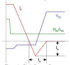
Figure 1c: Diode Reverse Recovery.
