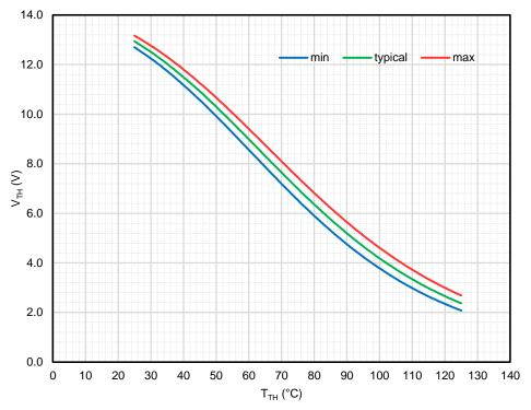
Figure 8:  $V_{TH}$  vs  $T_{TH}$  with  $V_{TH}$  pin pulled up to  $V_{CC}$  with a 7.50k $\Omega$  (1%, 100ppm) resistor. A 15V, 1% variation in V<sub>CC</sub> is assumed.
