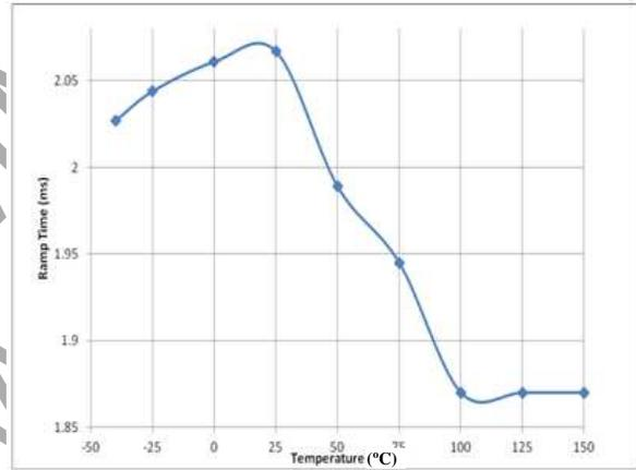
Figure 9. Output Voltage dv/dt Ramp Time vs. Temperature
