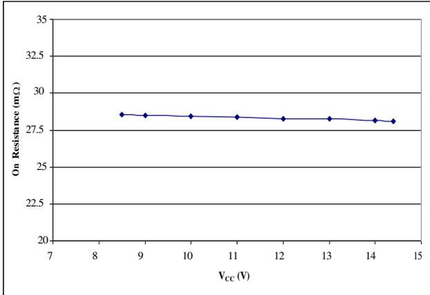
Figure 12. Power Device ON Resistance ( $R_{DS(ON)}$ ) vs.  $V_{CC}$
