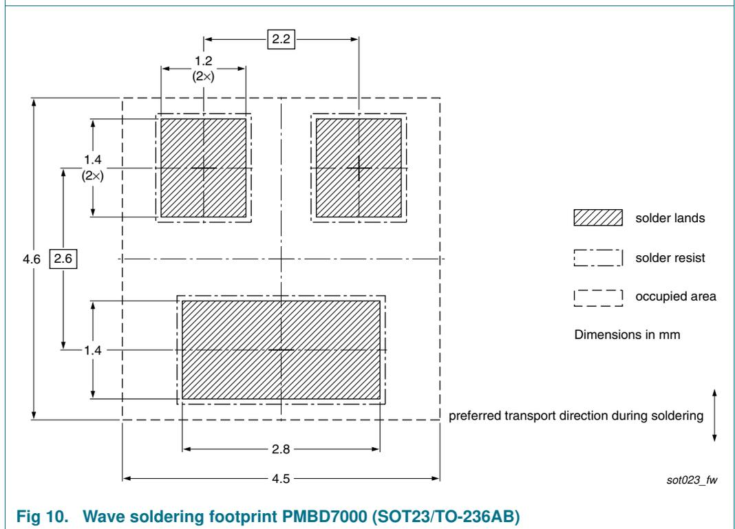
**Fig 10. Wave soldering footprint PMBD7000 (SOT23/TO-236AB)**
