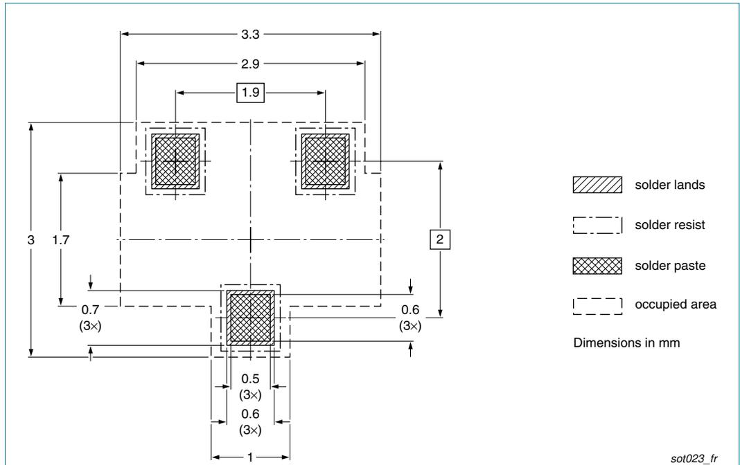
**Fig 9. Reflow soldering footprint PMBD7000 (SOT23/TO-236AB)**
