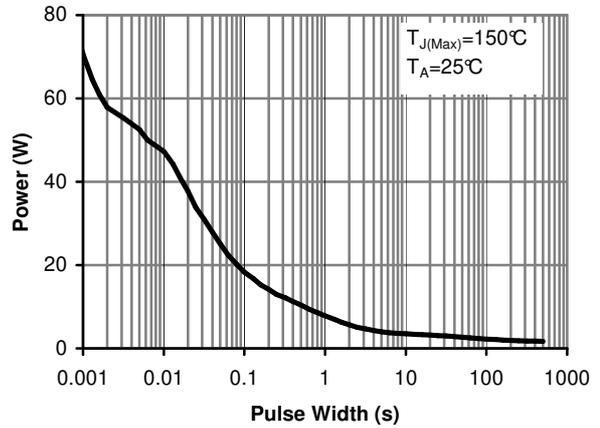
Figure 10: Single Pulse Power Rating Junction-to-Ambient (Note F)
