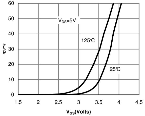
Figure 2: Transfer Characteristics
