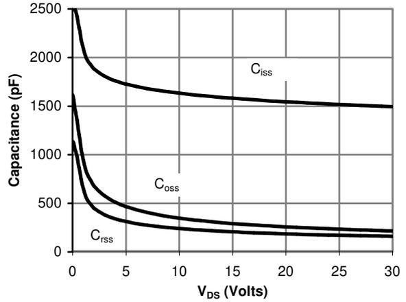
Figure 8: Capacitance Characteristics
