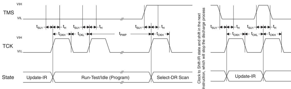
Figure 5-5. Verify Timing Diagram
