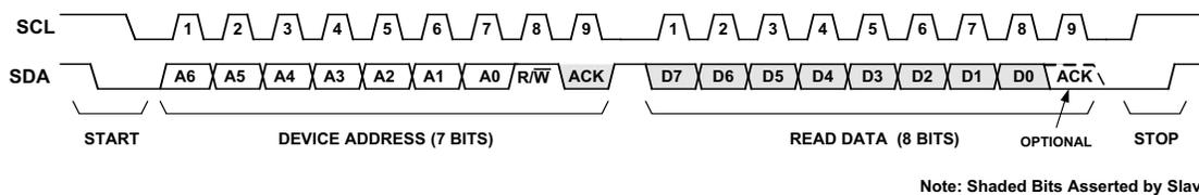
The LA-ispPAC-POWR1014ALA-ispPAC-POWR1014A provides 17 registers that can be accessed through its I<sup>2</sup>C interface. These registers provide the user with the ability to monitor and control the device's inputs and outputs, and transfer data to and from the device. Table 5-7 provides a summary of these registers.
