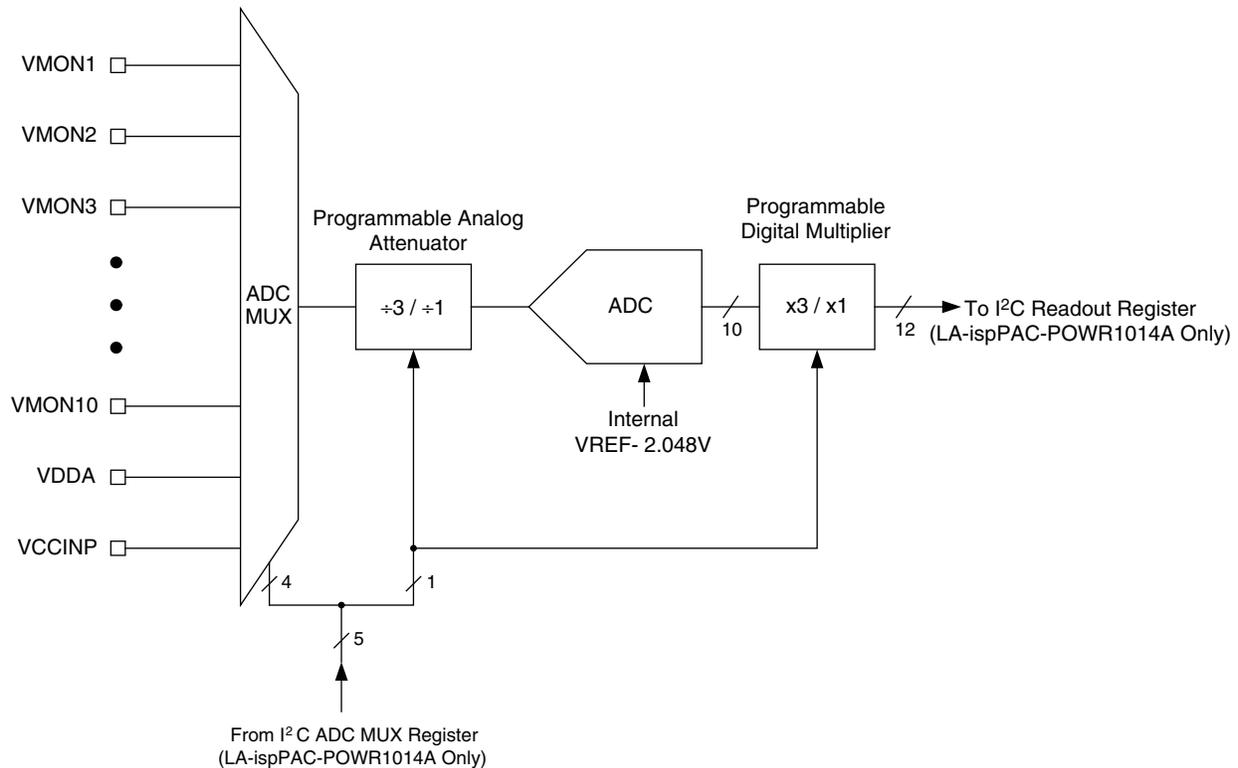
Figure 5-9 shows the ADC circuit arrangement within the LA-ispPAC-POWR1014A device. The ADC can measure all analog input voltages through the multiplexer, ADC MUX. The programmable attenuator between the ADC mux and the ADC can be configured as divided-by-3 or divided-by-1 (no attenuation). The divided-by-3 setting is used to measure voltages from 0V to 6V range and divided-by-1 setting is used to measure the voltages from 0V to 2V range.
