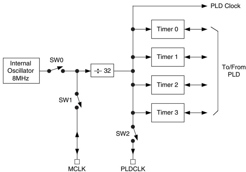
The internal oscillator runs at a fixed frequency of 8 MHz. This signal is used as a source for the PLD and timer clocks. It is also used for clocking the comparator outputs and clocking the digital filters in the voltage monitor circuits and ADC. The LA-ispPAC-POWR1014/A can be programmed to operate in three modes: Master mode,
