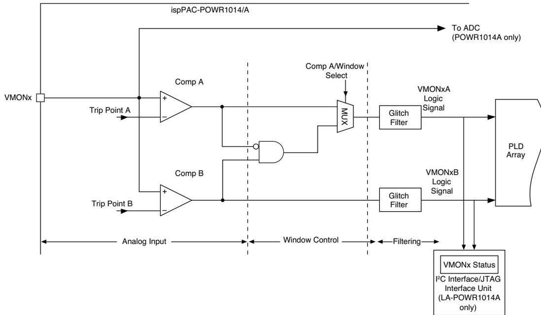
Figure 5-7 shows the functional block diagram of one of the 10 voltage monitor inputs - 'x' (where x = 1...10). Each voltage monitor can be divided into three sections: Analog Input, Window Control, and Filtering.
