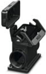
Box mounting bases B16, With single locking latch, Material: Polyamide, Protective cover material: Polyamide, Cable outlets: 2, Lateral, Height: 84 mm, Cable gland: none, Gland: no, 2x M40, Protective cover: Yes, Standard
