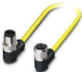
Sensor/actuator cable, 3-position, PVC, Plug angled M12 SPEEDCON, A-coded, on Socket angled M12 SPEEDCON, A-coded, cable length: 3 m
