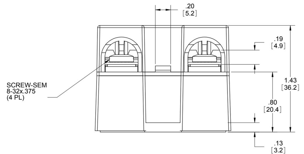
Tolerances:  $\pm$  0.02 in / 0.5 mm. All dimensions are in: inches [millimeters]
