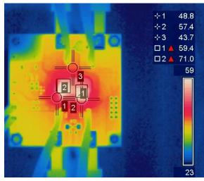
Figure 17: Thermal Image at VIN = 19V,  $I_{OUT}$  = 8A (IR3871: 71°C, Inductor: 59°C, PCB: 44°C)
