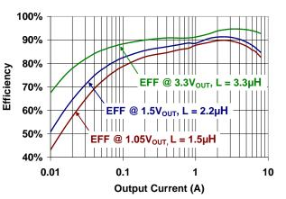
Figure 2. Efficiency vs. Output Current for VIN = 12V
