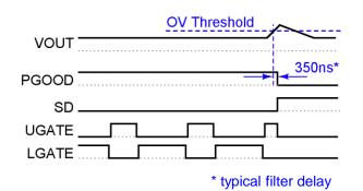
Figure 19(b). Over Voltage Protection
