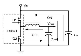
Figure 24. Current Path of Power Stage
