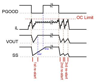
Figure 20. Over Current Protection
