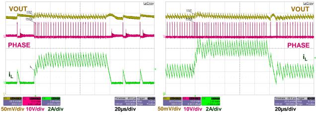
Figure 14: Load Transient 0-4A
