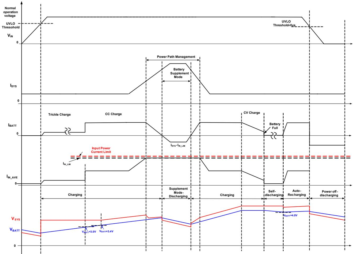
Figure 6— MP2625B Operation Process under No Fault Condition
