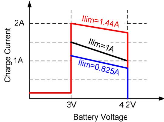
**Figure 7— $I_{CHG}$  Variation with Different Input Current Limit**
