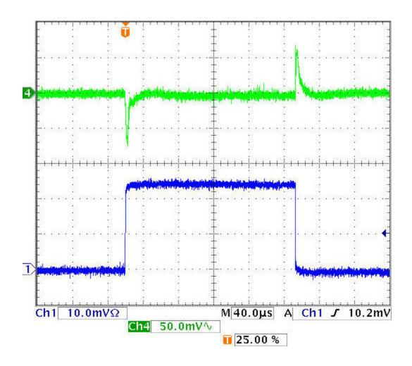
Figure 3. Load Step Response
