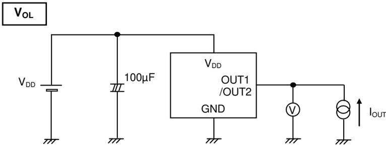
Figure 4. V<sub>OL</sub> Measurement Circuit
