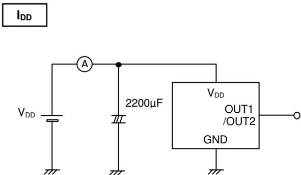
Figure 5. I<sub>DD</sub> Measurement Circuit
