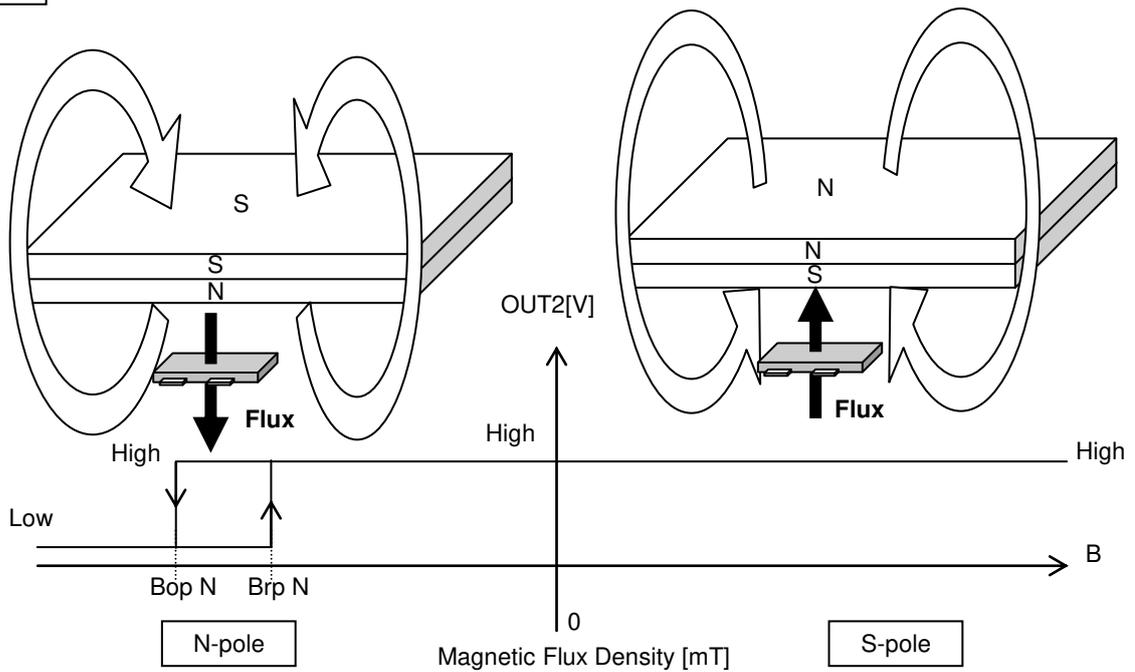
Figure 16. N-pole Detection
