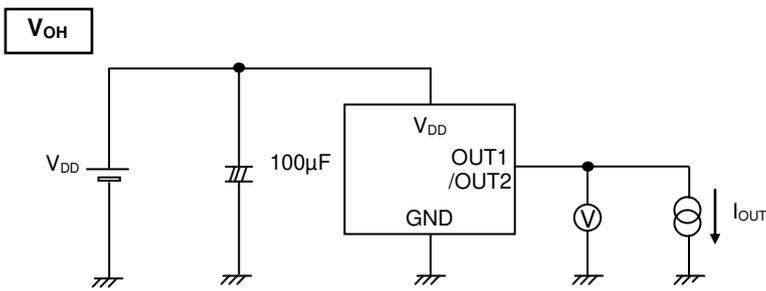
Figure 3. V<sub>OH</sub> Measurement Circuit
