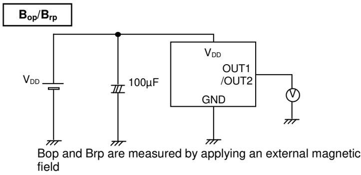
Figure 1. B<sub>op</sub>,B<sub>rp</sub> Measurement Circuit
