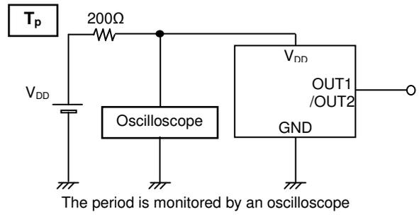
Figure 2. T<sub>p</sub> Measurement Circuit
