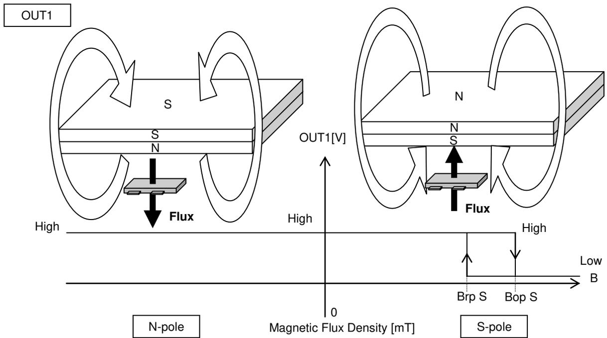
Figure 15. S-pole Detection
