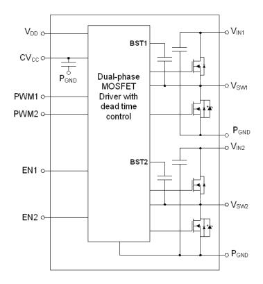
Figure 10 Internal Block Diagram
