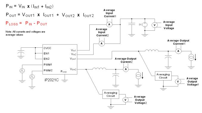
Figure 7 Power Loss Test Circuit
