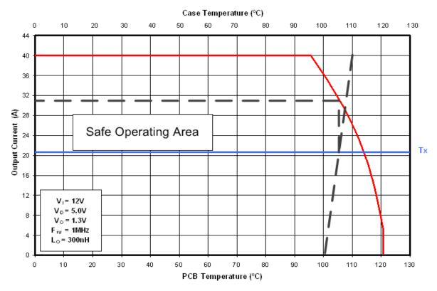
Figure 9 SOA Example, Continuous current  $\approx$  31A for T<sub>PCB</sub> = 100°C & T<sub>CASE</sub> = 110°C
