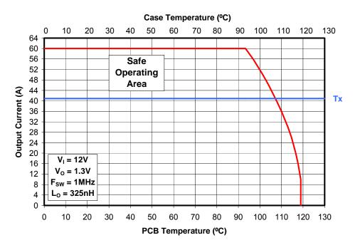
Figure 2 Safe Operating Area Curve
