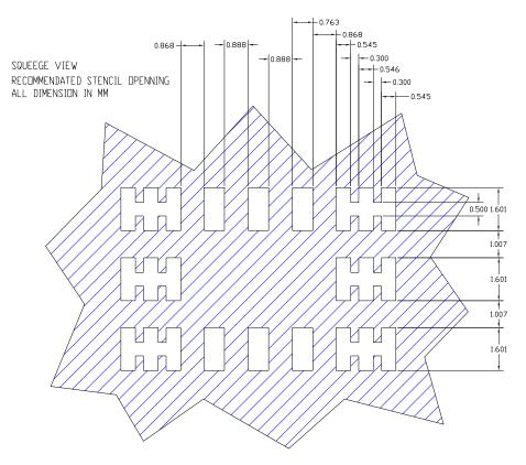
Figure 15 Solder Paste Stencil Design
