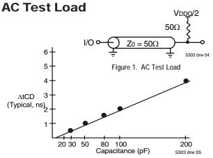
Figure 2. Lumped Capacitive Load, Typical Derating
