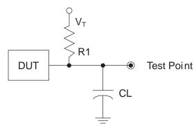
Table 3-1. Test Fixture Required Components, Non-Terminated Interfaces
