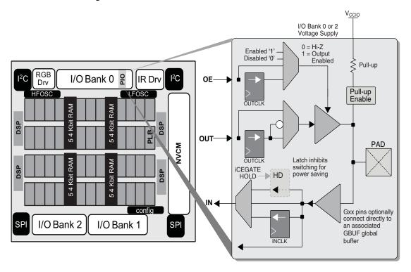
The PIO contains three blocks: an input register block, output register block iCEGate<sup>™</sup> and tri-state register block. To save power, the optional iCEGate<sup>™</sup> latch can selectively freeze the state of individual, non-registered inputs within an I/O bank. Note that the freeze signal is common to the bank. These blocks can operate in a variety of modes along with the necessary clock and selection logic.
