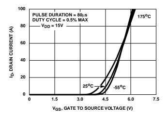
FIGURE 8. TRANSFER CHARACTERISTICS
