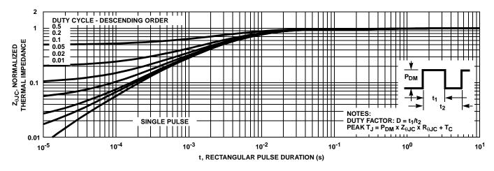
FIGURE 3. NORMALIZED MAXIMUM TRANSIENT THERMAL IMPEDANCE
