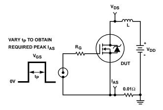
FIGURE 14. UNCLAMPED ENERGY TEST CIRCUIT
