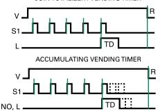
V = Voltage S1 = Initiate Switch NO = Normally Open Contact L = Load TD = Time Delay R = Reset
