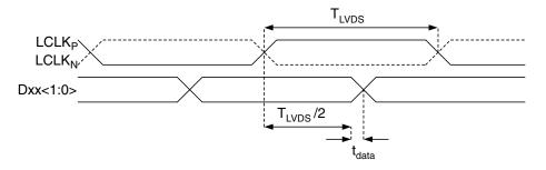
Figure 7. LVDS data timing, DDR mode
