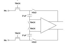
Figure 11. Input configuration
