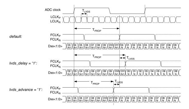
Figure 10. LVDS output timing adjustment
