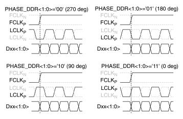
Figure 8. Phase programmability modes for LCLK
