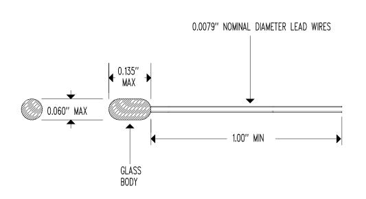
RESISTANCE @  $+25^{\circ}C = 50,000 \Omega \pm 10\%$ RESISTANCE/TEMPERATURE CURVE = "J" BETA " $\beta$ " (+25 TO  $+85^{\circ}C$ ) =  $3,977^{\circ}K$  NOMINAL TEMPERATURE COEFFICIENT @  $+25^{\circ}C = -4.4\%$ 'C NOMINAL DISSIPATION CONSTANT =  $0.7 \text{ mW/}^{\circ}C$  NOMINAL (AIR) THERMAL TIME CONSTANT = 5 SECONDS NOMINAL (AIR)MAXIMUM TEMPERATURE RATING =  $+300^{\circ}C$
