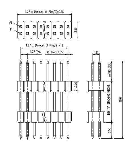
1. MATERIAL, HOUSING: HIGH TEMP THERMAL PLASTIC, UL94-VO
