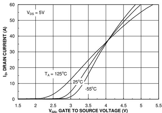
Figure 5. Transfer Characteristics
