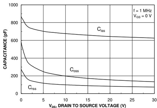
Figure 8. Capacitance Characteristics
