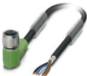
Sensor/actuator cable, 5-position, PUR halogen-free, black-gray RAL 7021, shielded, free cable end, on Socket angled M12 SPEEDCON, A-coded, cable length: 3 m
