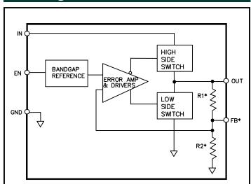
\* R1 and R2 are only in fixed voltage parts. FB pin is only present in adjustable part.
