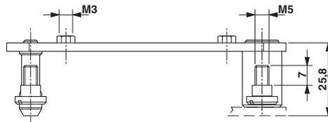
max. dimensions of both the docking frames (in case of standard contacts 25.8 mm;
