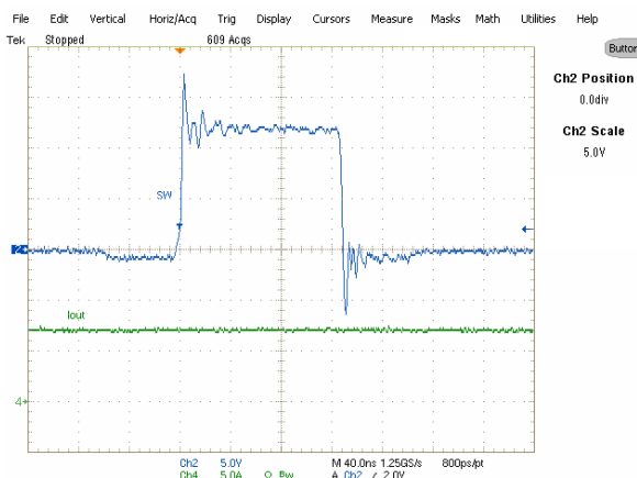
Fig. 11: Inductor node at 7A load, V_p: 0.6V , Ch2: LX , Ch4: I_{out}
