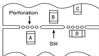
\*1  $A > D$  is valid when stress is added vertically to the perforation as with Hand Separation.
