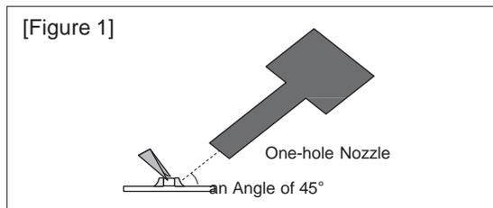
3. Optimum solder amount when re-working with a soldering iron
