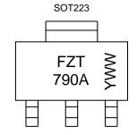
FZT 790A = Product Type Marking Code YWW = Date Code Marking Y or  $\overline{Y}$  = Last Digit of Year (ex: 5= 2015) WW or  $\overline{W}W$  = Week Code (01~53)
