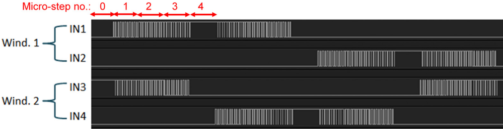
Figure 34. Logic Analyzer output
